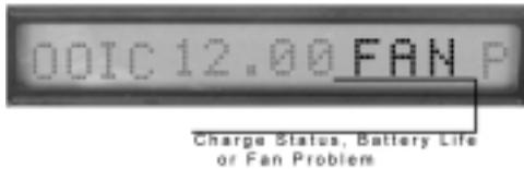
'Fan' - Indicates a Case Fan Problem The 'Fan' indicator alternates (about 3 seconds) with the Charge Status or Battery Life.
