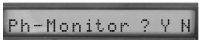
Press and hold the function button again, a blinking cursor will toggle between the **'Y'** and **'N'**. Release the function button and the system will save the current setting (about 10 seconds). This setting will remain in effect until changed, even if the unit is powered off. Clear the alarm using the function button **'C'** option.
